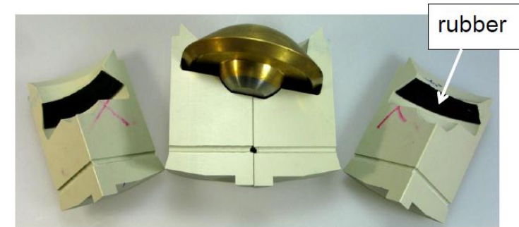
Model/sabot package for \alpha_0 = 10^\circ
