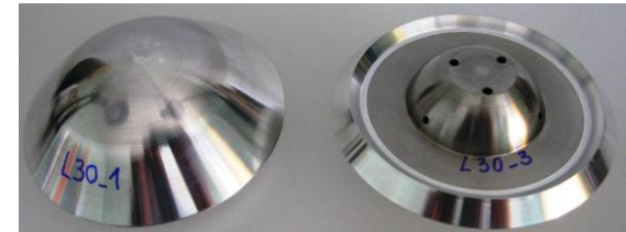
Model L_30 (tungsten/zircal: m=539 g) X_{cg}/D = 30\%
